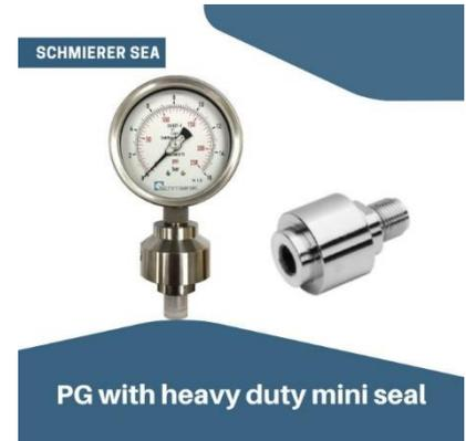
The diaphragm is AISI 316L welded to the body to ensure separation of the filling fluid from the process medium.
